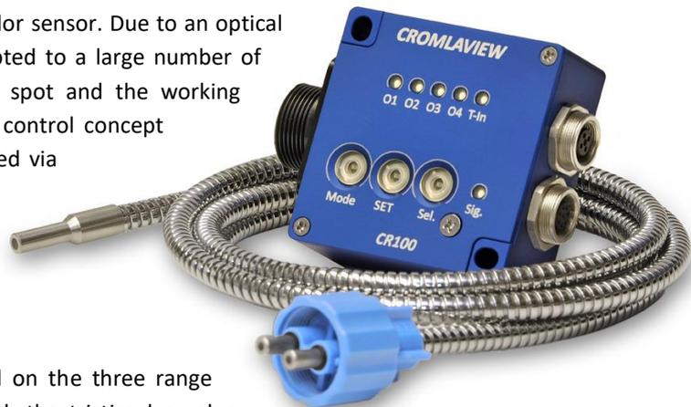
The functional principle of the CR100 is based on the three range procedure. The measuring light is assessed with the tristimulus value functions and assigned to the three wave length ranges red, green and blue. Through the assessment with these tristimulus value functions the sensor is able to perceive colors similar to the human eye.
