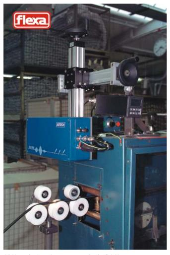
VLM 200 A - Length measurement for the finishing process
